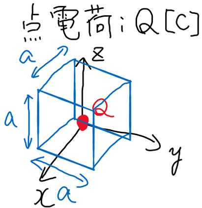
$$\begin{aligned} \iiint_V \rho dV &= \int_{x=-a/2}^{a/2} \int_{y=-a/2}^{a/2} \int_{z=-a/2}^{a/2} Q \delta(x) \delta(y) \delta(z) dx dy dz \\ &= Q \underbrace{\int_{x=-a/2}^a \delta(x) dx}_{=1} \underbrace{\int_{y=-a/2}^{a/2} \delta(y) dy}_{=1} \underbrace{\int_{z=-a/2}^{a/2} \delta(z) dz}_{=1} \\ &= Q \text{ [C]} \end{aligned}$$
